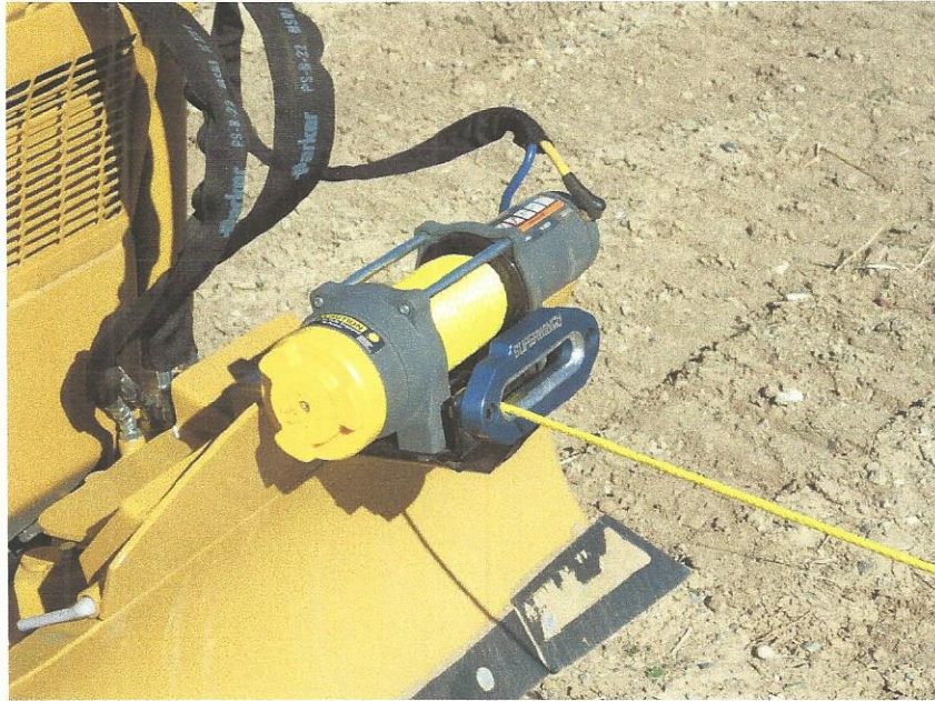
Winch – 4500 lb. 12 volt with synthetic rope, 2/Hawse fairlead Front Mount
